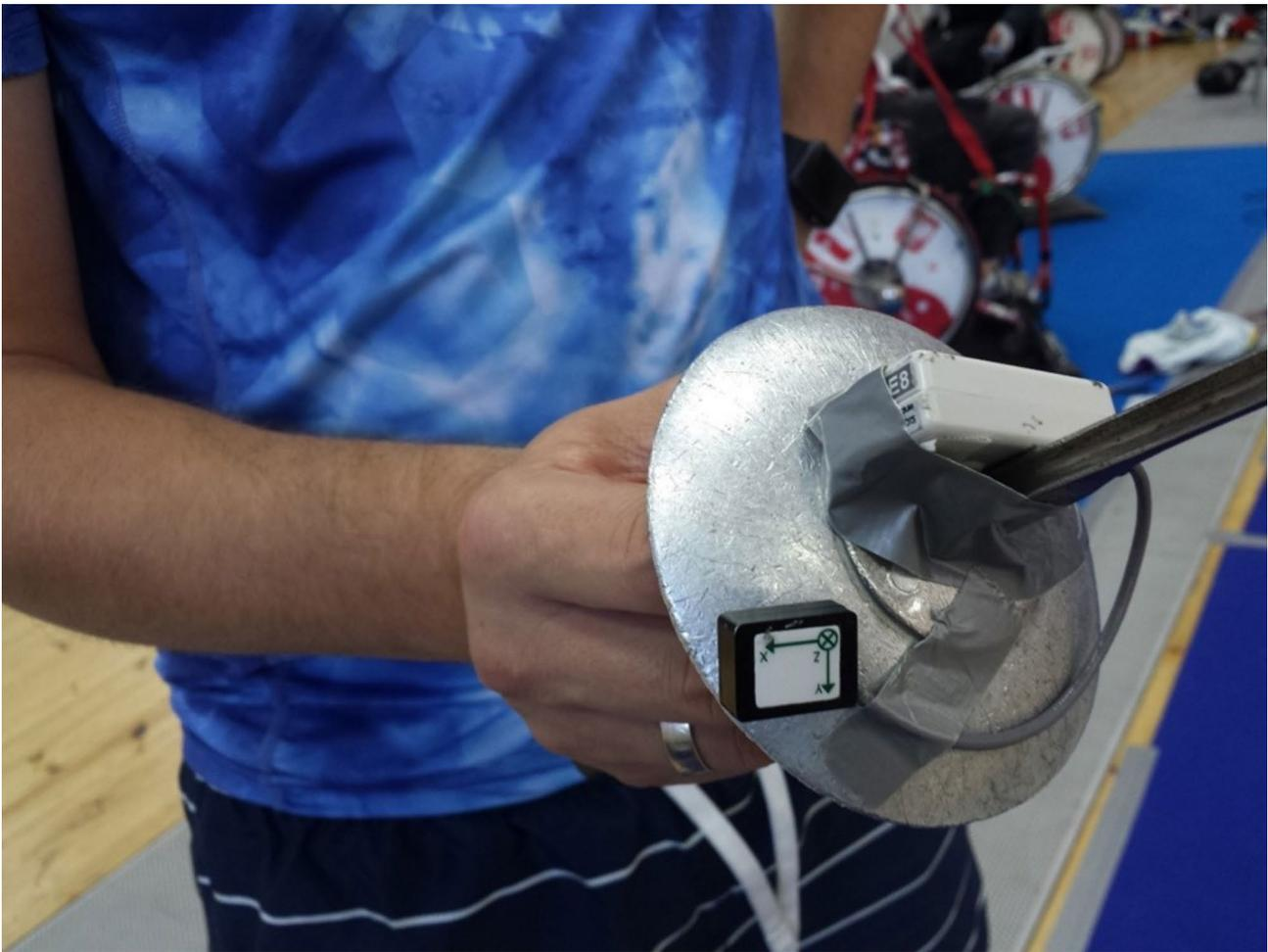
**Fig. 1** Preparation of the trainer's weapon with attached accelerometer
